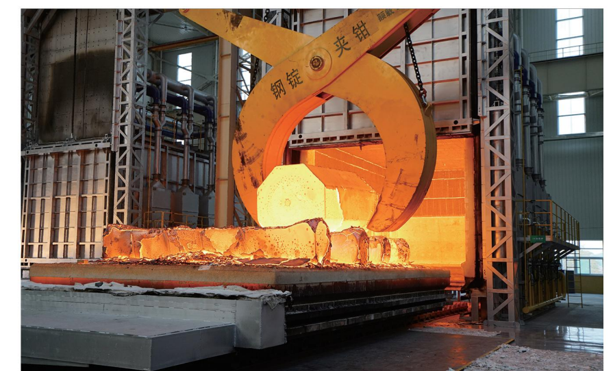
炉膛宽度8米台车式加热炉 Trolley type furnace with furnace width of 8 m
